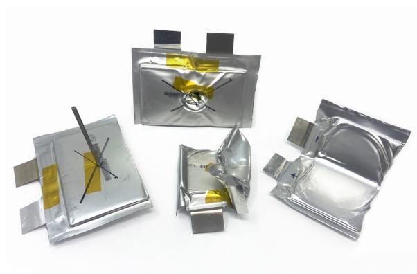
Figure 12 SVolt 5 Ah NMC811/graphite cells that have been mechanically abused without going into thermal runaway (left). The cell discharge curve taken on nail penetrated cells four hours after they were damaged, showing more than 90% retained capacity. The mechanical abuse in the cells on the left forms the basis of the mechanical abuse in the Soteria Safety Standard.
